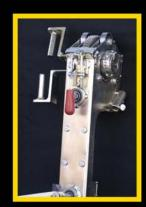
STEP 3: Slide the winding fingers separately into the drum & position the drum assembly over the garage door shaft and cone. Slide the drum back together.
