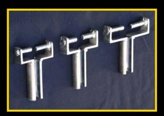
Note that the SpringTurner can be set up for right hand springs and left hand springs.
